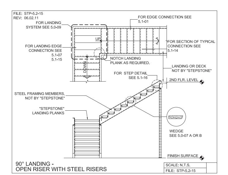
PRECAST CONCRETE TREADS AND LANDINGS SHOWN ON PLANS SHALL BE FROM THE LONG SPAN "STEPTREAD" SYSTEM BY "STEPSTONE, INC." OF GARDENA, CA FOR STEEL CONSTRUCTION. THE MANUFACTURER IS TO SUPPLY ALL PRECAST CONCRETE "STEPTREAD" SYSTEM PARTS, FEATURING BOTTOM WELD PLATES FOR WELD-ON CONNECTIONS. ALL REINFORCING AND CONNECTION PLATES WILL BE ZINC PLATED. ONLY ITEMS NOTED AS BY "STEPSTONE, INC." WILL BE FURNISHED BY "STEPSTONE, INC." SUCH ITEMS ARE TO BE INSTALLED BY OTHERS.
